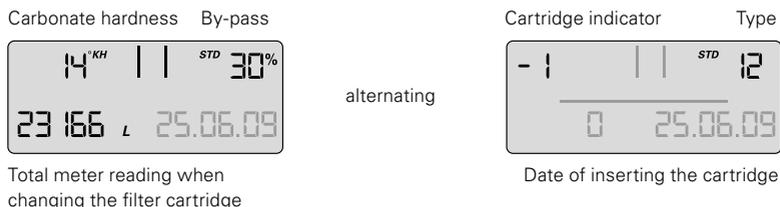
At the top left, the indicator for the filter cartridge (-1 for previous filter cartridge) is displayed alternately with the carbonate hardness set and the hardness unit. At the top right, the filter system size is displayed alternately with the by-pass setting (display 1 s indicator, 1 s carbonate hardness), at the bottom left, the meter reading when changing the cartridge (-1) and at the bottom right, the installation date of the cartridge.
